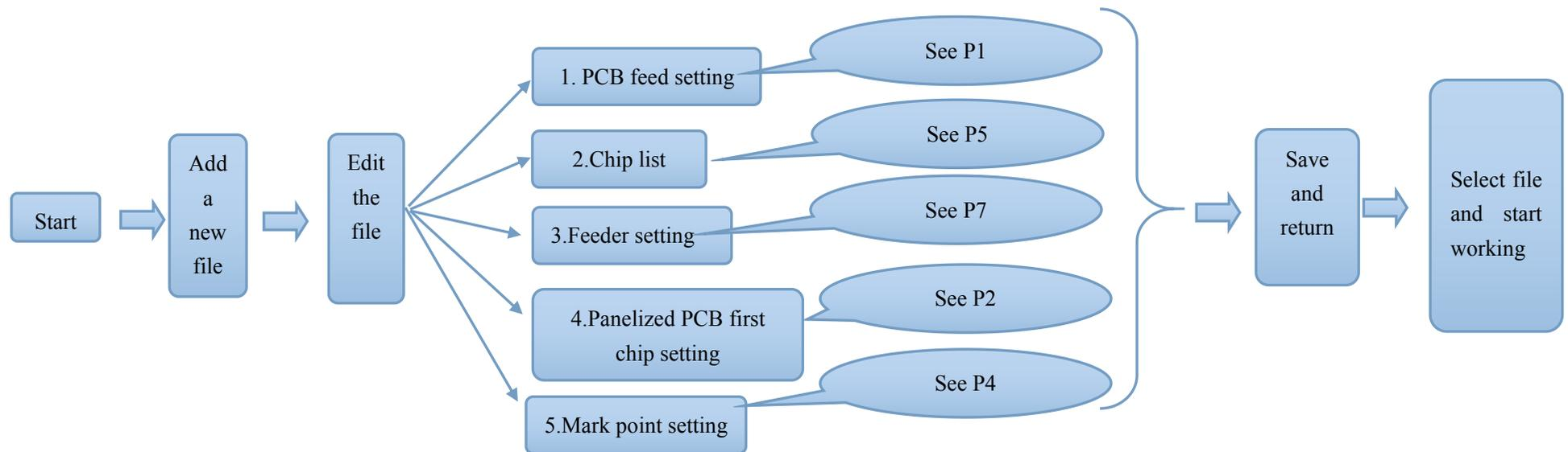
Note: The basic procedure of making a programming file for manual programming or direct PCB file is similar, but there are two different parts: chip list and mark point setting. Please find the detailed operation steps of the differences on relative page.
