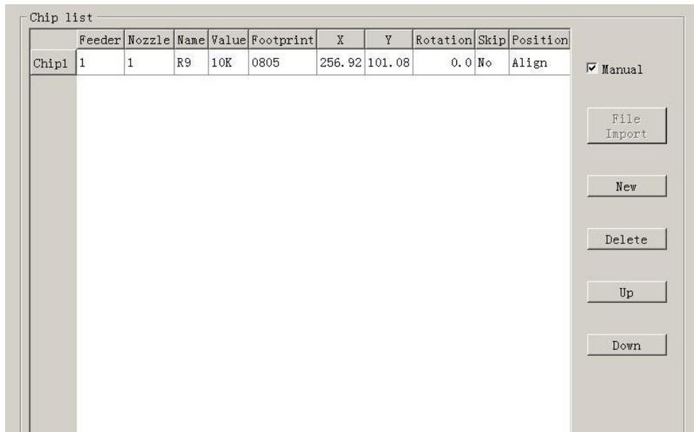
Function: to display the sequence, footprint and other information of components. There are two ways to add these information: manual programming and import mounting file.
