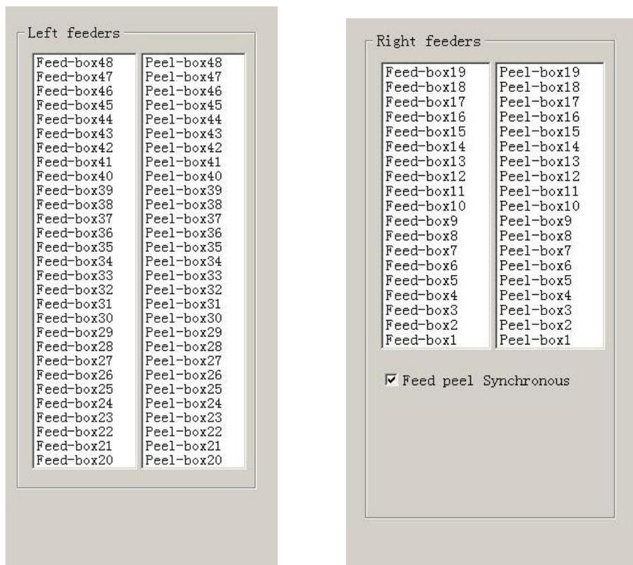
Function, test each feeder's matching and feed box & peel box's function. First, select "Feed-box and peel-box linkage", then test function of feed box and peel box.
