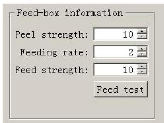
Function:Adjust the value for feed and peel box
