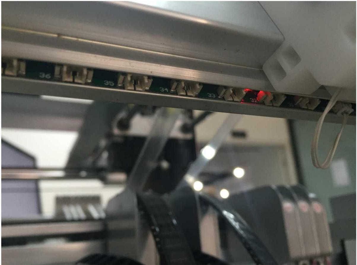
For example, the default port ID for Stack 33 is 33, if the port 33 is broken and want to change to port 34, can set in this item
