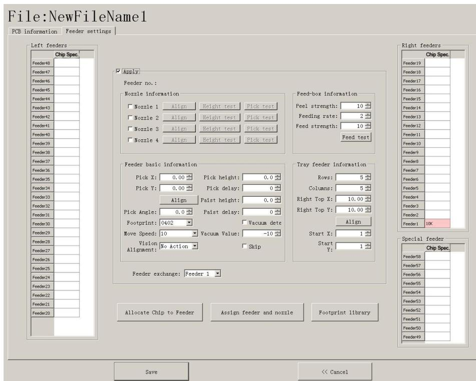
Functions: All components' configurations will be set here for every working file, i.e. (Nozzle selection, Feeder selection, Pick up position, Correction setting and other parameters)
