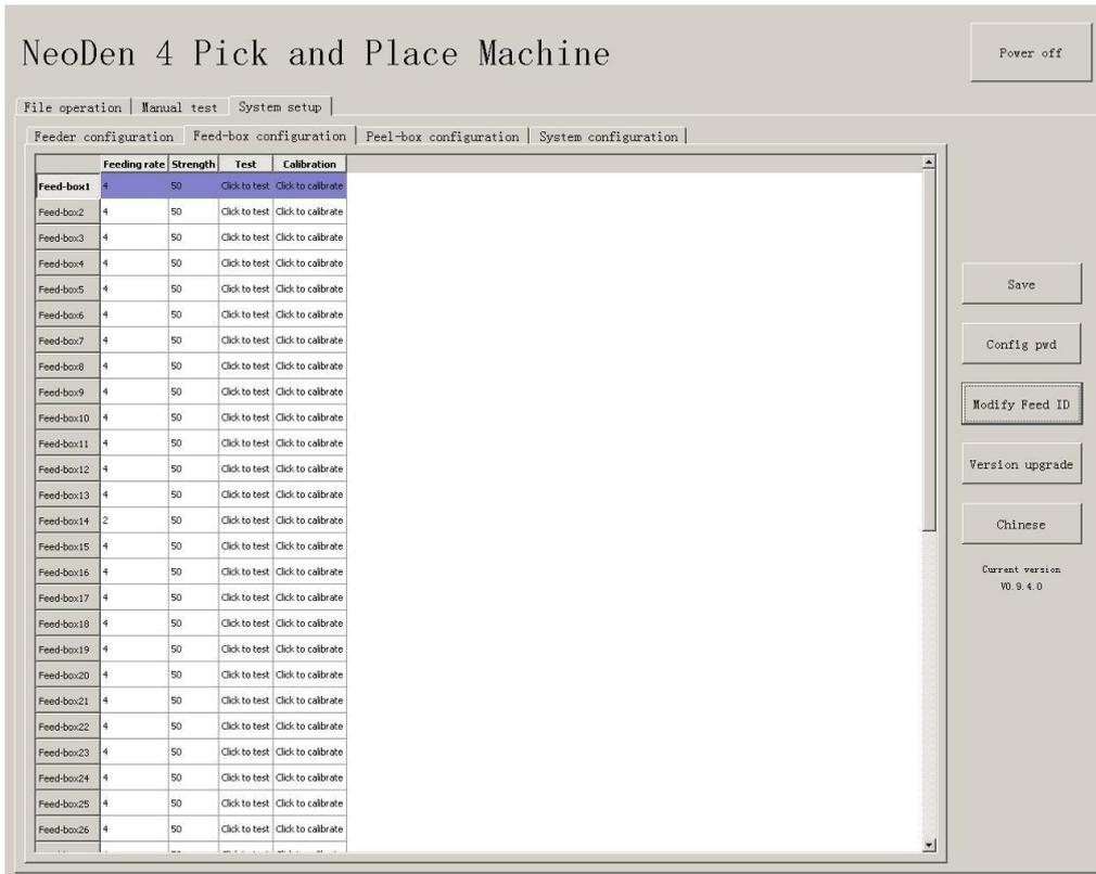
Function: Peel configuration as above figure show, used to set the values for all peel boxes
