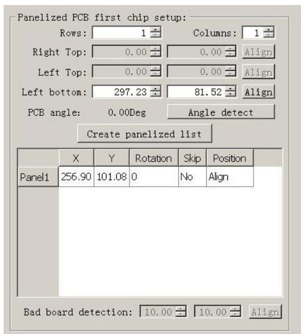
Function: This is mainly to determine the first component on single or panelized PCB of manual programmed or imported file. The principle is to collect and calculate the data of each board's relative spacing, in order to achieve the effect of the actual placing.
