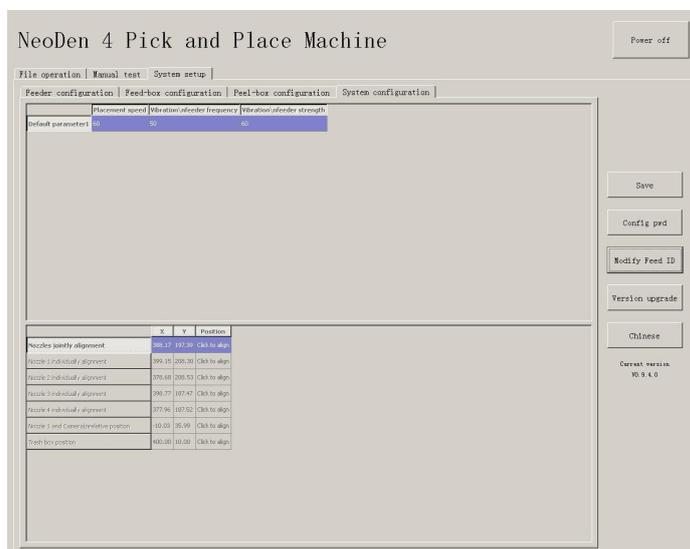
Function: it is mainly for correction the position of suction nozzle.(Notice: In case change by mistake,we 've locked it by password. It can be changed by clicking the button of Password change and then insert password. Strongly recommend operating it under our engineer ' s guidance).
