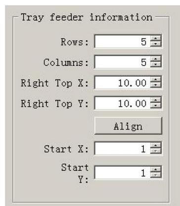
Function: Use to set the components' information from tray and tube packages, complete picking up operation for special feeders by changing the values
