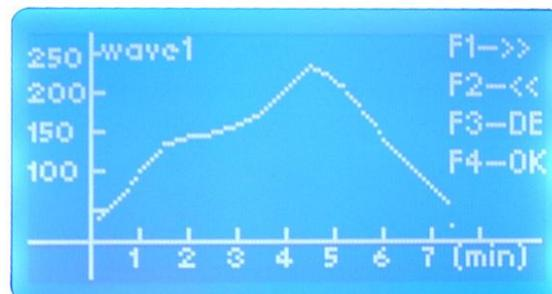
② Following we provide eight different waves, please choose one according to your request. Press the F1/F2 to choose different wave, press F3 to look into different wave parameter, press 4 to confirm the wave you chose.
