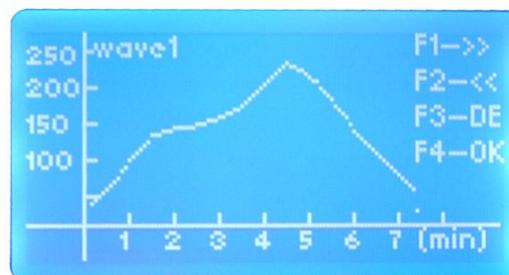
Press “F3” button again to see the parameters for the chosen wave, for example soldering paste sort, soldering temperature, time etc.
