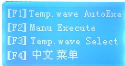
In the main menu, press the “F3” button to select different temperature waves. This example shows wave one:
