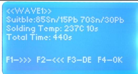
Press the “F4” button to return previous page. Press the temperature wave that the”F1” key carries out to make selection automatically, the process will shut down automatically upon completion and a warning buzzer will sound.
