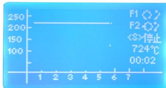
Press “F1” button to start cooling, Press F1/S key again to stop. Press “F2” button to start heat up, Press F2/S key again to stop.
