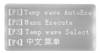
In the main menu, press the "F3" button to select different temperature waves. This example shows wave one:
