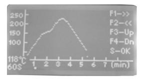
Press "F1/F2" button, forward and backward to select different time. Press F3/F4 button up and down to select different temperature, Press "s" button to save.
