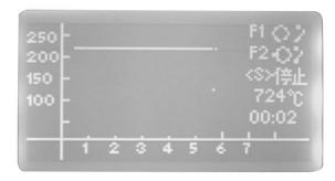
Press "F1" button to start cooling, Press F1/S key again to stop. Press "F2" button to start heat up, Press F2/S key again to stop.
